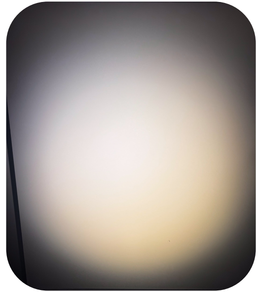
An example of poor CoA performance, in which the bottom-right portion of the beam appears significantly more yellow/amber than the rest of the beam.
