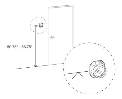
Junction box must be mounted precisely 50.75" - 56.75" (on center) above the finished floor surface to ensure compliance with **ADA Standards.**
