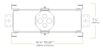
\*Can be field cut to minimum 7 1/2" (191mm)
