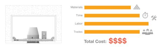
Although this is an effective method, it requires the ceiling space to have boxed-out cavities, using the same fire-resistance rated membrane material, to mount the recessed fixtures in. This approach adds significant costs and requires extra space above the ceiling plane that may not always be available.
